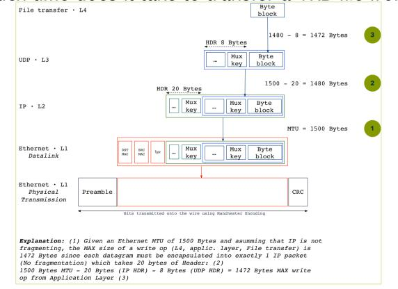
Assume an Ethernet segment connects two end stations, A and B which are located at a distance of 2500 m from each other. How much time does it take to transfer a 1KB file from A to B?
