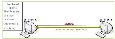
Assume an Ethernet segment connects two end stations, A and B which are located at a distance of 2500 m from each other. How much time does it take to transfer a 1KB file from A to B?
